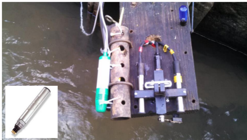
Figure 3: Turbidity/FDOM sensor mounted on a board immersed in the water. The image in the corner is a Turner Designs Cyclops-7 submersible sensor.
