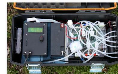
Portable 3-chamber Soil Respirometer
