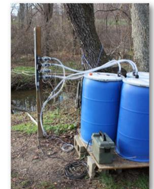
The Dial-a-Pump controller operates a bank of large solenoid valves in order to fill multiple barrels for sampling the stream water during different parts of a storm.
