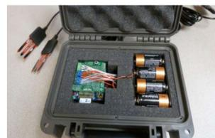
6-channel soil moisture probe logger: \$60
