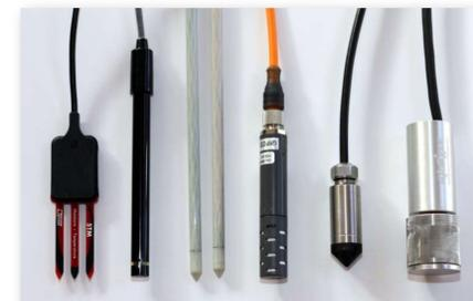
Some of the commercial sensors that can easily connect to Arduino loggers: soil moisture, conductivity, redox, CO<sub>2</sub> probes, pressure transducers, and oxygen sensors. These are the same sensors used with commercial dataloggers, so we can collect the same high-quality data with our custom loggers.
